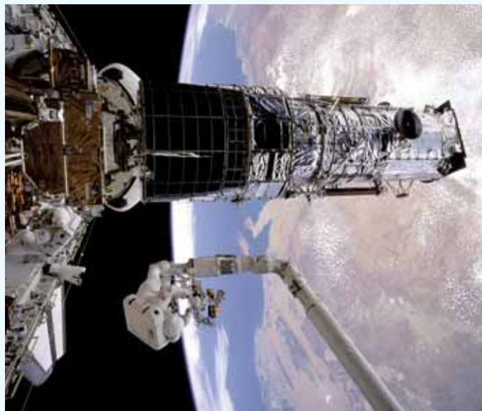
THE HUBBLE SPACE TELESCOPE has enjoyed a long, successful life because it was designed to be serviced by shuttle astronauts. NASA
